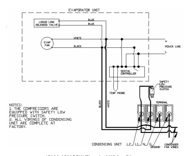
1500& 2500SSW Electrical Wiring Diagram
